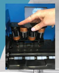
Load the batteries into the battery holder &place in the housing, clicking it into place
