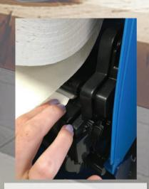
Place the end of the roll between the rollers
